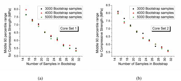
Fig. 8 – Middle 90 percentile range of compressive strength of concrete: Variation with different number of data in each sample, (a) Core Set 1, (b) Core Set 2
