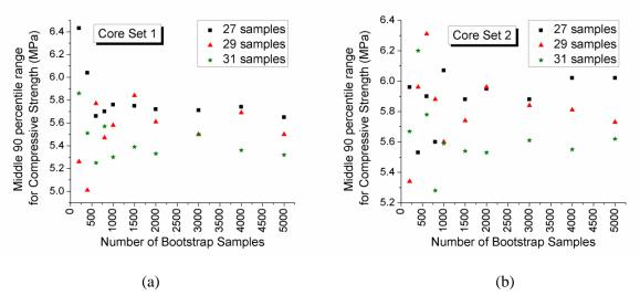
Fig. 7 – Middle 90 percentile range of compressive strength of concrete: Variation with different number of bootstrap samples, (a) Core Set 1, (b) Core Set 2
