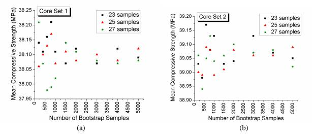
Fig. 3 – Mean compressive strength of concrete: Variation with different number of bootstrap samples, (a) Core Set 1, (b) Core Set 2
