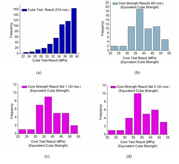
Fig. 1 – Histograms: (a) Original cube results, (b) core results, (c) Core Set 1, (d) Core Set 2
